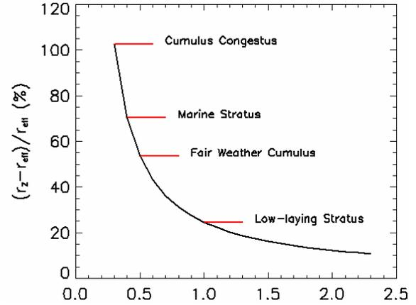
Fig. 3. Percent error between effective radius,  $r_{eff}$ , and the radar reflectivity based estimate of cloud drop size,  $r_z$ , calculated based on the modified gamma drop-size distribution and cloud parameters tabulated in Ulaby et al. (1981) and the marine stratus distribution shape observed by Vali (1998).
