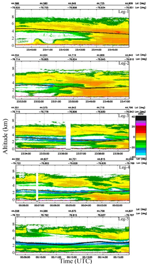
Fig. 7. Sequences of vertical profiles of  $Z$  measured by the zenith and nadir-looking W-band radar along a S-N track, while doing porpoise maneuver between 2.5 km and 4 km. The back line shows the aircraft altitude.
