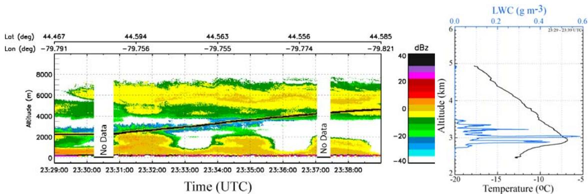
Fig. 5 Left: Vertical Profile of W-band Z measured by the NAWX zenith and nadir-looking antennas during the spiral ascent in a multi-layer cloud system. The aircraft altitude is shown by the black line. Right: vertical profiles of T (black) and LWC (blue) measured during the spiral ascent.
