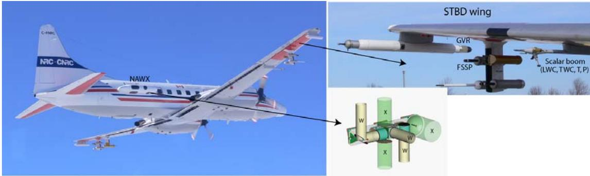
Fig. 1. During the C3VP field project, the NRC Convair-580 aircraft was equipped with an array of in-situ Cloud Physics instruments mounted in under-wing and wing-tip pylons. Schematics of the NAWX antenna configurations in the blister radome and the in-situ probes mounted on the starboard side of the aircraft including the GVR installation on the wingtip are shown in the picture.
