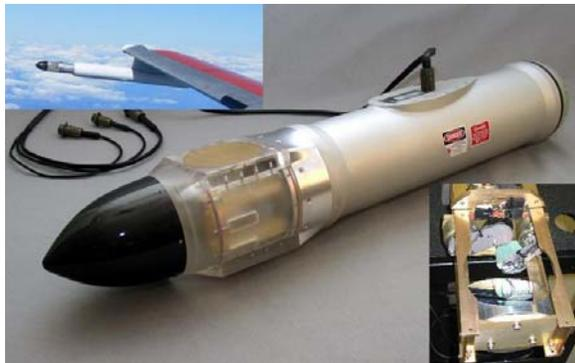
Fig. 2. Airborne GVR installed on the NRC Convair-580 aircraft (upper left), in a standard PMS probe canister (middle) and with the radome head removed, showing the fixed 90 degree metal mirror and the solenoid
