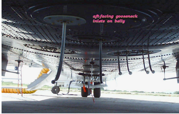
Figure 1. Belly of C-130 shows assortment of gooseneck inlets, antennas, and other instruments
