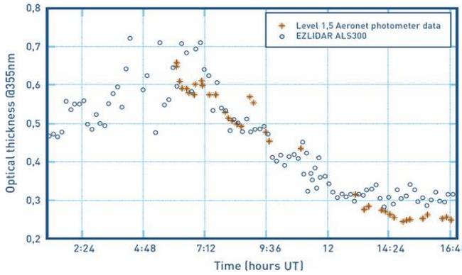
Figure 2 Level 1.5 Aeronet photometer data (red) AOD EZLIDAR retrieval (blue)
