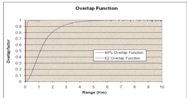
Figure 4 EZLIDAR(red) and MPL(blue) overlap function
