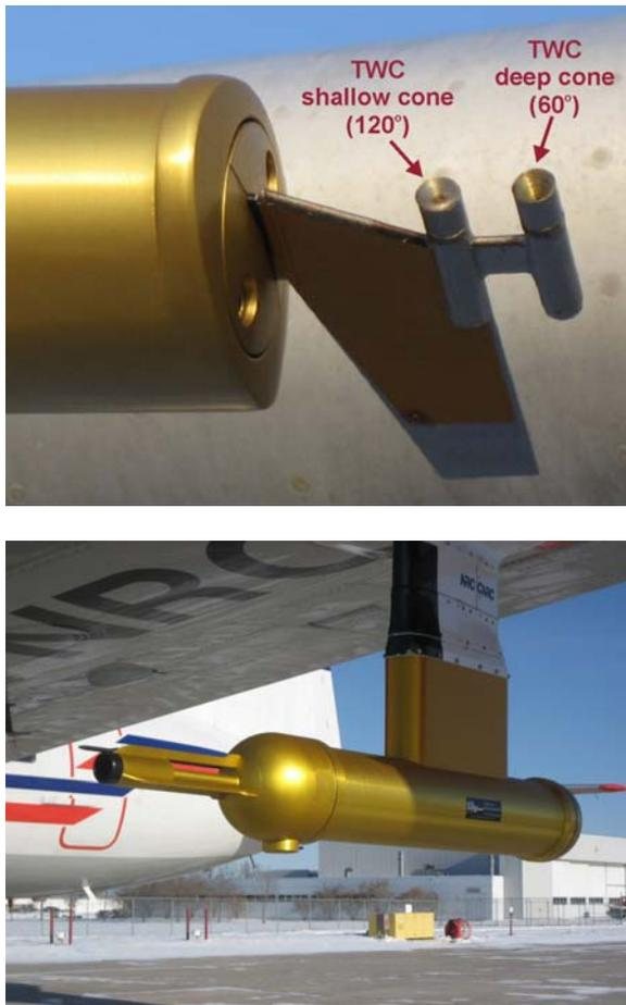
**Figure 6.** Modified Nevzorov sensor head; both shallow and deep sensors mounted on the same vane (top). DMT CVI probe installed on the NRC Convair-580.
