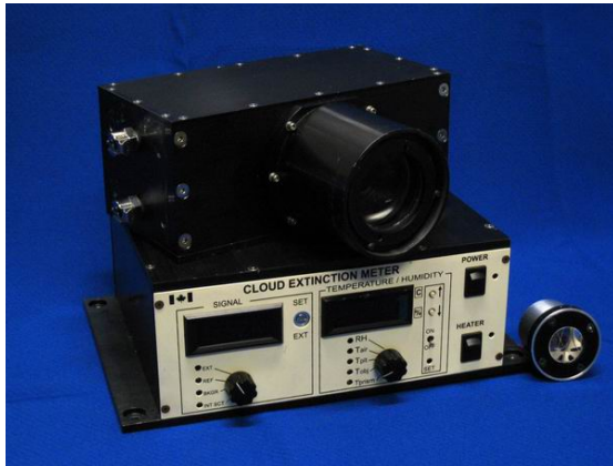
Figure 3. Cloud Extinction Probe: optical unit (top); control box (bottom); retroreflector (right).
