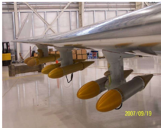
Figure 2: Modifications to be able to carry instrument canisters under the wings.
