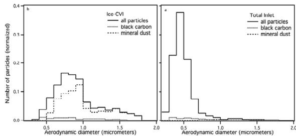
**Fig.6:** Comparison of mass size distributions of background aerosol (total inlet) and ice particle residues (Ice-CVI) measured with the ATOFMS.
