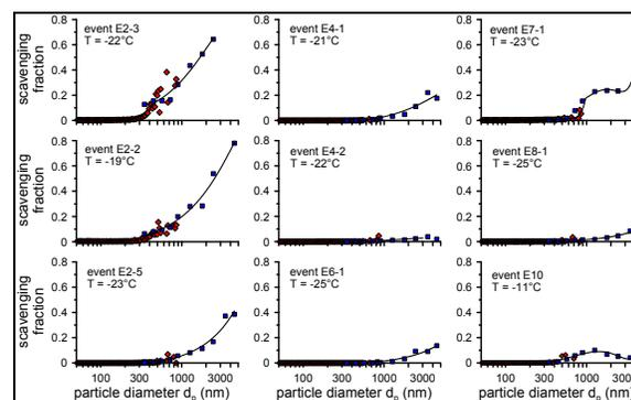
**Fig.2:** Scavenged number fractions of IN as a function of their particle size. Diamonds (red) and squares (blue) present SMPS and OPC measurements, respectively.
