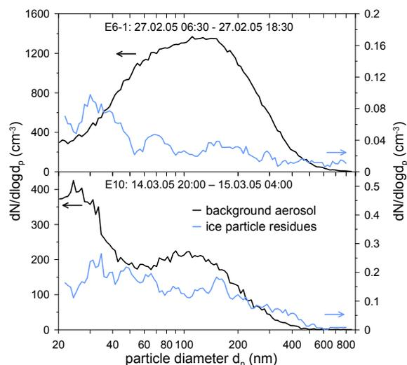
**Fig.1:** Mean background aerosol (black line) and ice particle residue (blue line) number size distributions measured with two scanning mobility particle sizers (SMPS). The latter is linked to the right y-scale.
