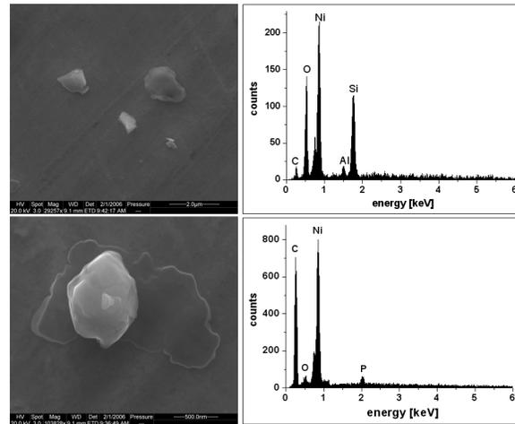
**Fig.7:** Secondary electron image and EDX spectrum of ice particle residues. The Ni peak is caused by the substrate.
