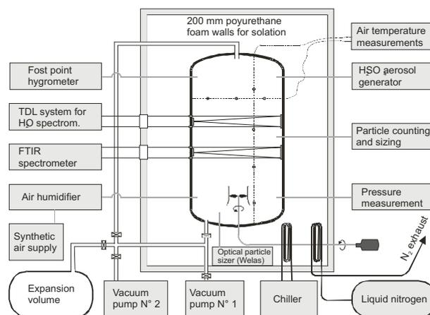
Figure 1: Schematic view of AIDA facility with key instrumentation
