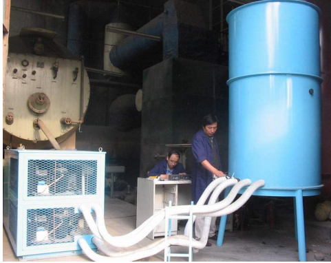
Fig.1. A photograph of 1m 3 Isothermal cloud chamber (ICC) in CAMS
