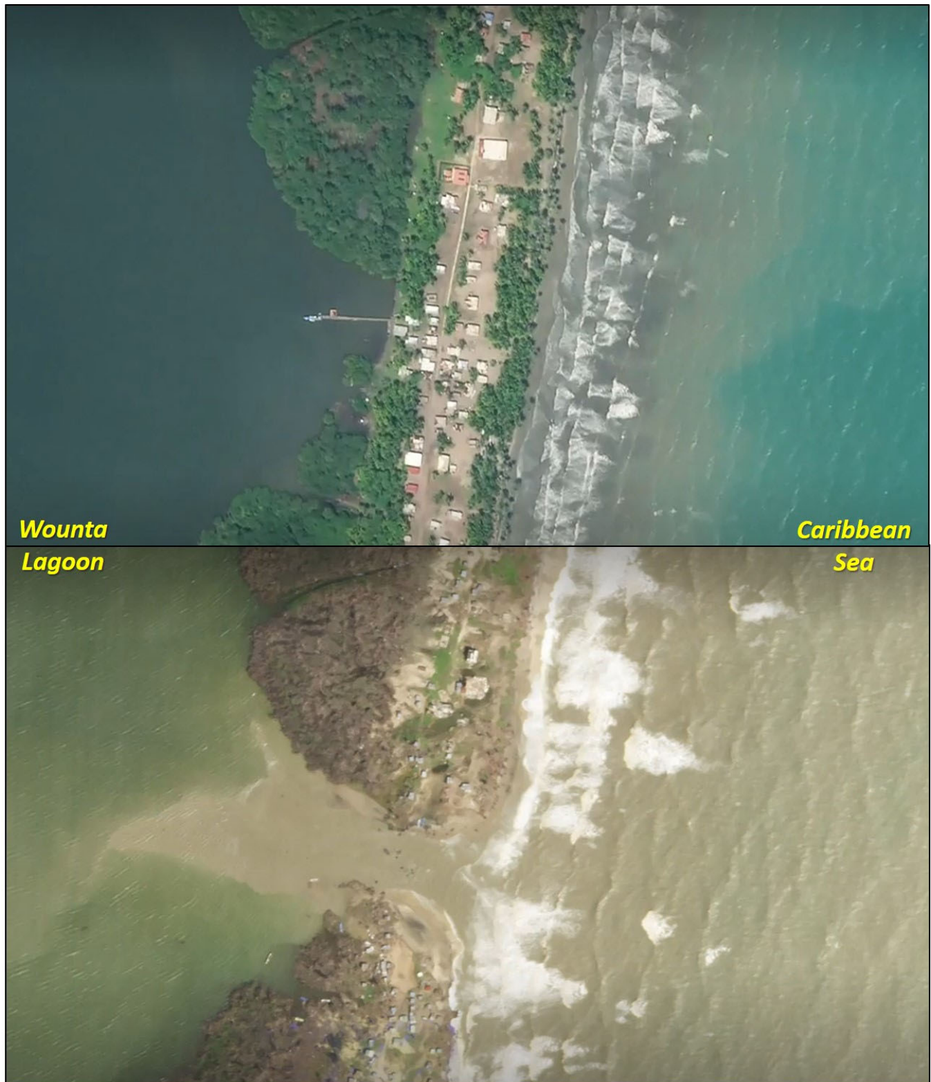
Figure 17. Before (top) and after (bottom) overhead pictures depicting erosion of the barrier island and the development of a cutout caused by Hurricane Iota's storm surge at Haulover, Nicaragua, on 17 November 2020. (images courtesy New York Times )
